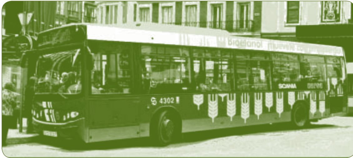
Diesel cycle bus fuelled with hydrated ethanol in Madrid.
