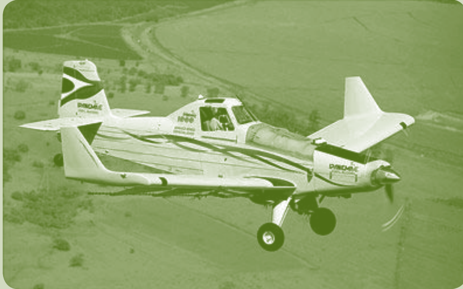
Embraer Ipanema: a hydrated ethanol agricultural plane.
